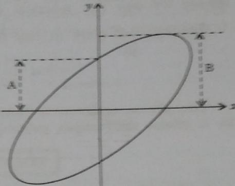
Fig. 2.6-4 : Measurement of phase differences
