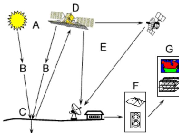
**1. Energy Source or Illumination (A)** - the first requirement for remote sensing is to have an energy source which illuminates or provides electromagnetic energy to the target of interest.
